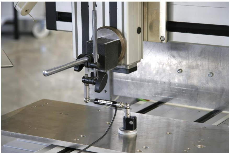
Picture: circular form measure with Renishaw QC10
