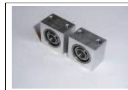
Part No. 919D30 Bearing Blocks. 5mm I.D. (19.06 x 19.0mm x 10mm) Part No. 919D30/1 Bearing Blocks. 6mm I.D. (15.87 x 19.0mm x 12.5mm) Part No. 919D30/2 Bearing Blocks. 8mm I.D. (19.0 x 19.0mm x 13.0mm)
