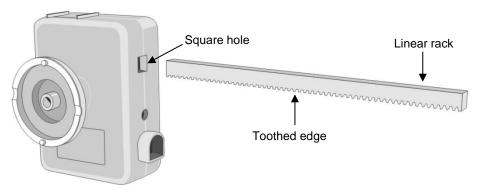
The linear rack fits into the small square hole that can be found on both sides of the Rotary Motion Sensor. Insert the linear rack gently into the hole (from either side) with its teeth pointing downwards (towards the shaft of the pulley wheel). Feed in the rack until it just emerges from the square hole on the other side.
