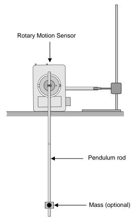
The length of the pendulum is defined as the distance from the point of suspension to the centre of gravity of the bob. To find the centre of gravity, place the pendulum rod/mass rod on a 'knife' edge and find the point at which it is balanced. Measure the distance from the point of suspension to the centre of gravity and use this value to give more accurate results.
