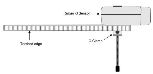
**Note:** Make sure that the clamp does not tighten onto the teeth of the rack.
