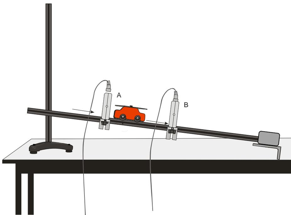
This diagram shows a typical apparatus set up for use with Timing. Light gates are connected to Input **A** and **B** on data logger and are used to monitor the movement of a cart down a track. An interrupt card is fixed to the top of the cart and this card will cut through the Light gate's infrared beam.
