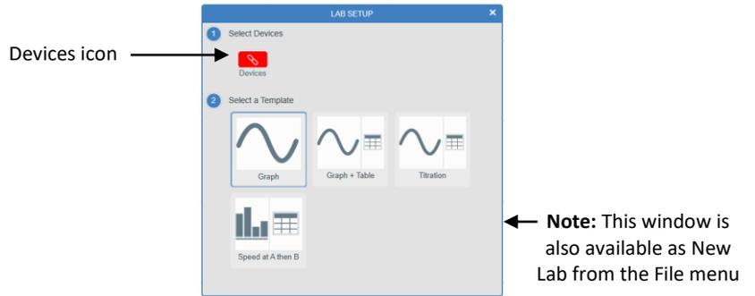
2. Select the data logger or wireless sensor from the list of available devices.
