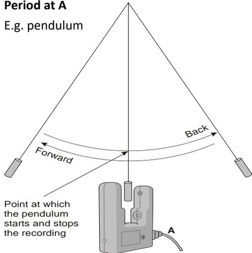
Start the pendulum swinging, when it is moving freely click on the **Start** icon.
