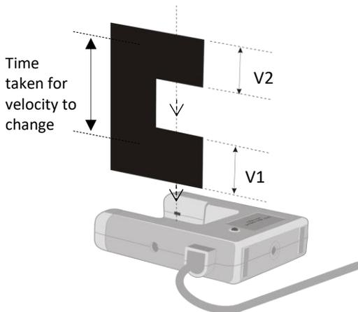
E.g. Average acceleration can be measured using a single Light Gate with a double interrupt card. Acceleration is calculated using the length of the segments on the double interrupt card.
