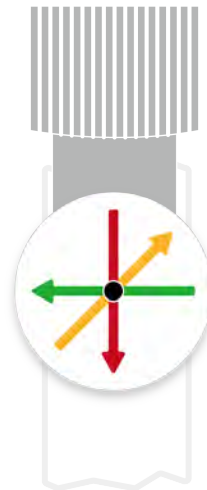
The moving paths of the laser spots on the double-sided tape on the laser head outlet.
