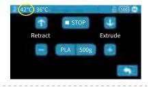
5 Gently press the end of the filament into the extruder inlet and push it to the end. When the temperature of the nozzle reaches the preset temperature, the printer will beep and the extruder will automatically grab the filament, and pull it in and extrude it through the nozzle.
