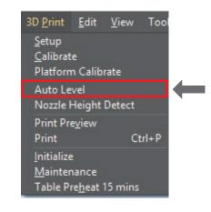
Install the UP Flex print board on the build platform, start the Auto Level function. Require UP Software 2.18 or later.
