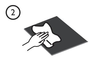
Clean the surface of UP Flex print board to remove any grease and dust.
