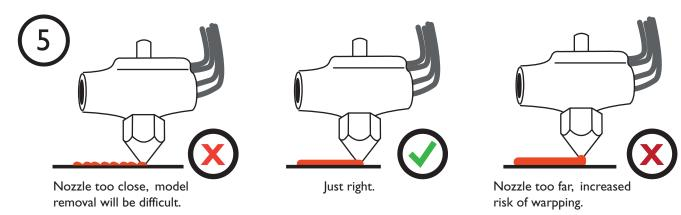
Make a test print, see how the raft is sticking to the surface. If the raft is sticking too well or too loose, adjust the nozzle height value manually at maintenance or print confirmation window.
