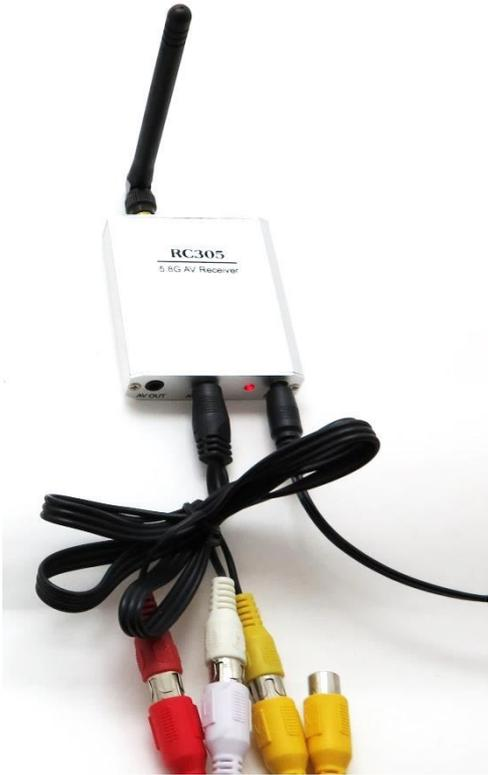
A photograph showing the RC305 5.8G AV Receiver with its antenna attached. The power cable is plugged into the DC/IN port, and the audio cable is plugged into the AV OUT port. The power adapter is also visible.                                                                                             |
