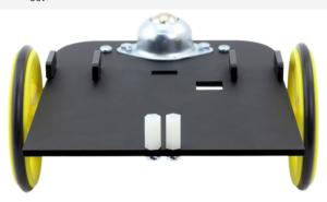
Mount the line following board to the spacers using two M3 x 6mm screws.
