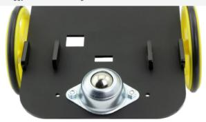
Attach the M3 x 20mm plastic spacers using two of the M3 x 6mm screws from underneath.
