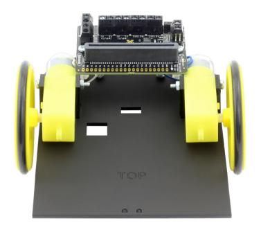
Take the wires from the motors and connect them to the terminal blocks on the motor driver board in the following configuration:
