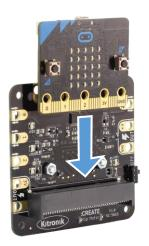
Power is provided via the integrated battery supply (3 x AA, ~4.5V), and the board then produces a regulated 3.3V supply which is fed into the 3V and GND connections to power the connected BBC micro:bit, removing the need to power the BBC micro:bit separately.
